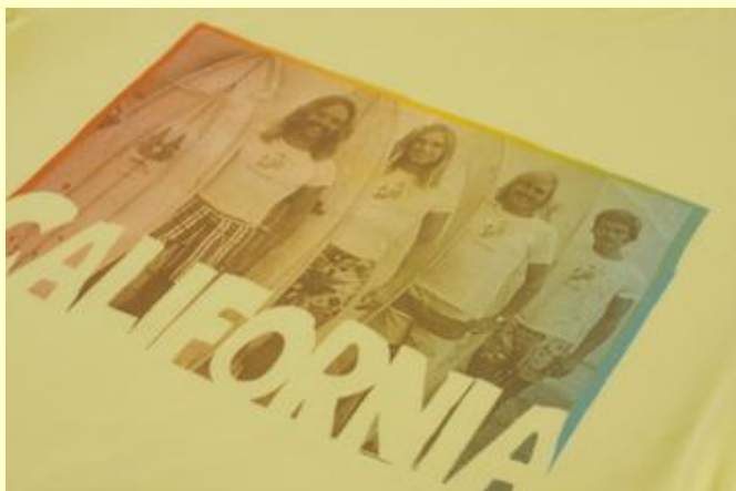
Printing with 180/inch, 48 micron, S-thread
