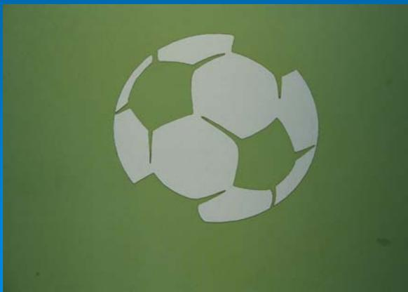
16. The stencil now needs to be dried with a cool air fan and/or limited heat until the screen is dry, then prepare it for the press.
