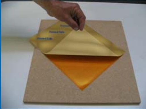
1. Remove clear printed protective layer to expose film surface for adhesion.
