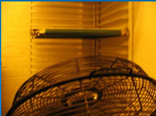
9. Place frame in a drying rack. Dry with either heat or cool air fan. When initial emulsion layer is dry, the frame is ready for final coating.
