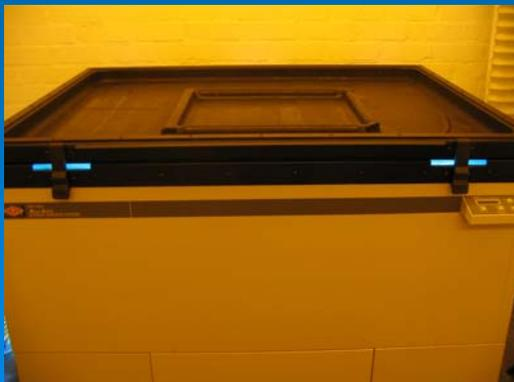
13. Expose the dried stencil. Exposure time with a 5kw metal halide lamp at 40" is approx. 1.5 minutes per 100 microns of film.
