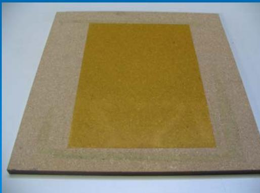
3. Place the Thick Film on the build-up board with the thick film emulsion facing up and the clear protective sheet against the build up board.
