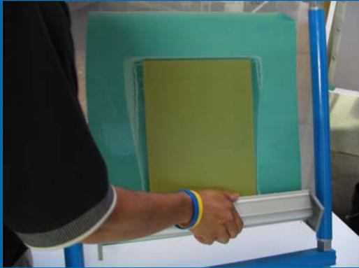
10. Coat squeegee side twice with the dull edge of the coater to seal the stencil. Dry completely until backing sheet releases with ease.
