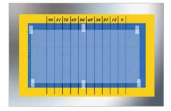
In the example shown, the screen will be exposed 10 times at 9 seconds for each exposure. Your time may vary depending on your exposure unit. Attach the blockout media as shown in the next graphics Expose the screen ten times using the Individual Panel Exposure as determined in the previous section. Move the rubylith, amberlith, or thin cardboard over one row for every exposure. Make sure not to move the positive
