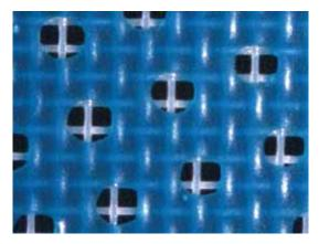
Halftones will show good edge definition with no over exposed emulsion blocking the small partial openings in the mesh.
